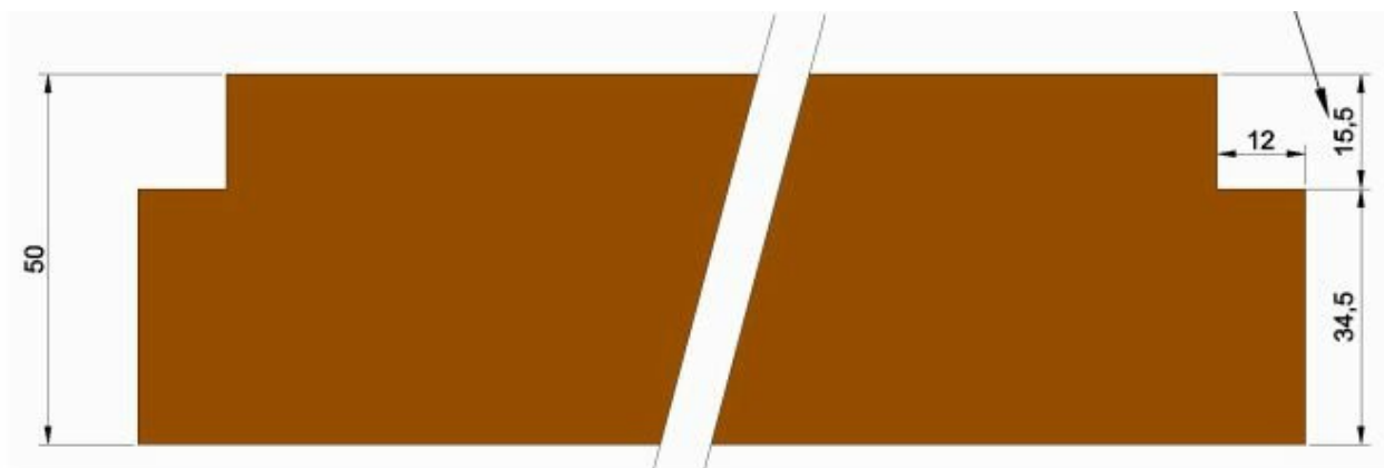
rebate dimension for 5mm door seal
